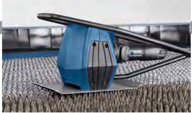
Figure 2. This electric slat cleaner uses two serrated tools that move up and down while oscillating as they pass over the slag. They scrape each side of the slat, clearing the hardened material. On flatbed laser machines with a pallet changer, the slag can be removed without losing any production time by clearing the slag from one table while the laser is in operation.
