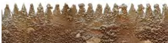
Figure 1. If slag accumulates on the support slats, the molten material has no space to go and the part will weld back into place, meaning the cut may be lost or parts may appear burnt or discolored and require a secondary process to restore an acceptable edge. The "kick back" or spatter from the cut may deposit on the parts, resulting in scrap. Spatter could also contaminate the laser lens, reducing cut quality or damaging the lenses or cutting head.
