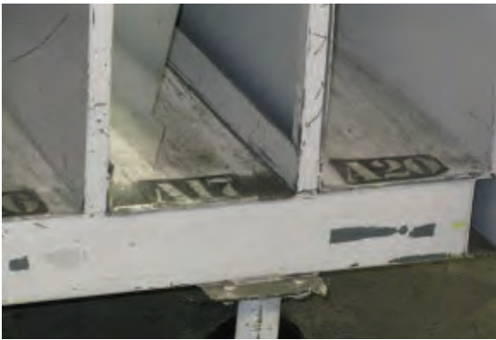
Figure 4 Part and part family numbers are marked at the bottom of individual slots. This means even new workers know where to place finished parts. It also makes it immediately apparent if a part is missing for an assembly.
