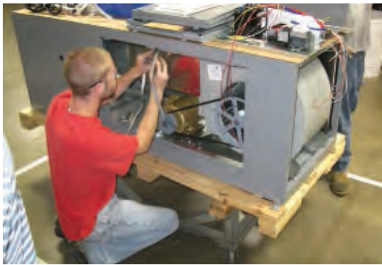
Figure 7 Final assembly workers produce eight units a day. After significant 5S efforts, stations have been organized, and tools can be seen on boards, not buried in individual toolboxes.
