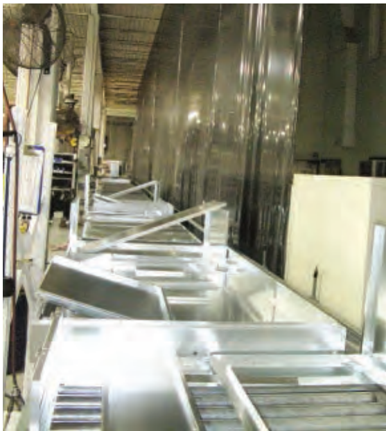
Figure 6 In the batch-processing days, workers would send batches of the same part down the conveyor, which spans the length of the prebuild department, which puts together subassemblies for downstream operations. Now they group different parts together, so workers downstream can retrieve all the parts they need for a subassembly in one kit.
