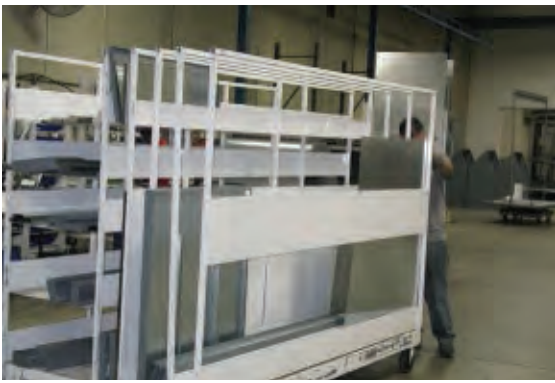
Figure 3 These custom carts make single-piece part flow possible. They carry every sheet metal part for each heater unit.
