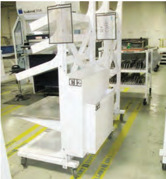
Figure 5 This cart holds parts that require forming, as well as the job jacket detailing the tools and precise setup needed for each component. Tools placed on a separate cart can be wheeled where needed. All this helps reduce wasted motion and shorten setup time.
