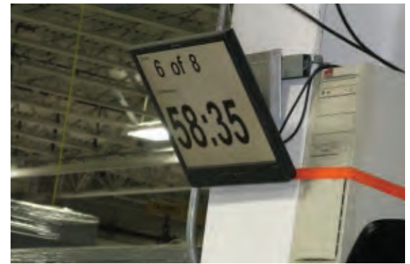
Figure 8 This clock counts down the takt time and shows the current status. At this point in the shift, workers had assembled six of the eight units for the day.
