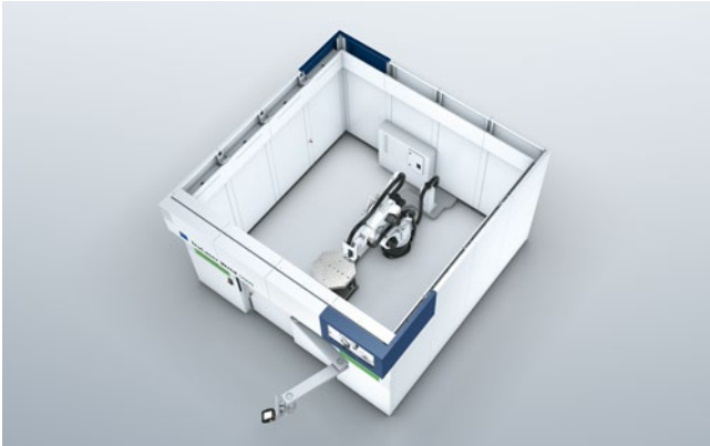
The rotate-and-tilt positioner enables you to weld even hard-to-access parts in a single clamping setup.
