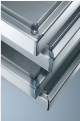
Mild steel terminal box (from bottom to top): unwelded, manual MAG weld, FusionLine weld, and laser weld after redesigning for laser processing.
